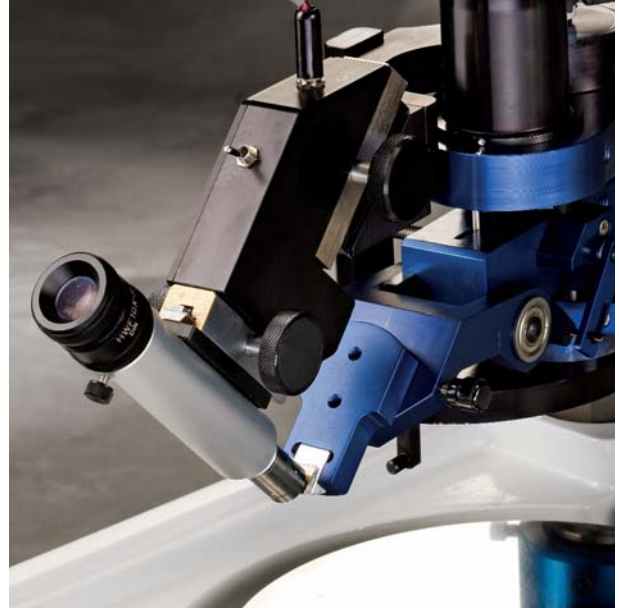
Bare die sample is easily aligned with the Tilt Alignment Microscope Accessory.
