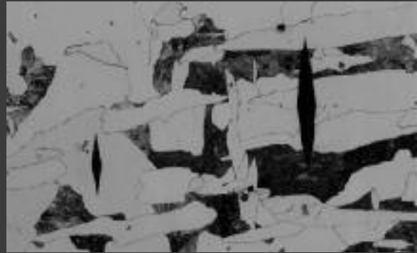
1045 Steel, etched with Nital, 25g and 50g Knoop (200x).
