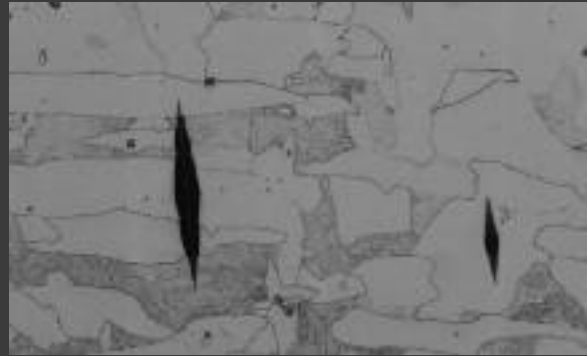
Replica of 1045 Steel, etched with Nital, 25g and 50g Knoop (200x).
