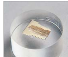
TransOptic™ Powder produces clear mounts
