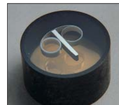
EpoxiCure™ has low shrinkage and hard mounts
