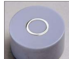
VariDur™ has a 10 minute cure time and high hardness
