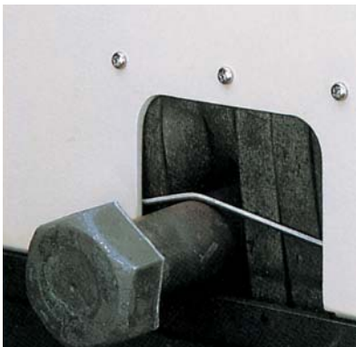
Rubber sealed side ports allow sectioning of long stock.
