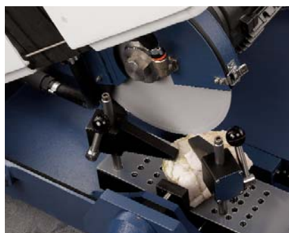
Rock Clamp Assembly with specimen.
