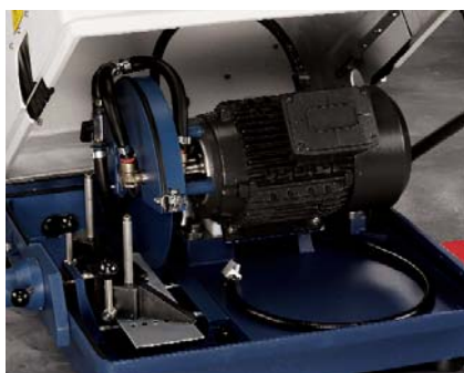
Delta® PetroCut™ Cutter showing Rock Clamp Assembly and Clean-out Hose.
