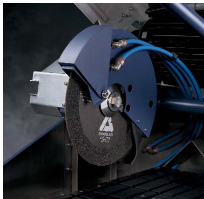
Wheel guard pivots open for easy wheel changing.
