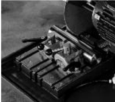
Sliding Vises are versatile quick release vises for routine clamping.
