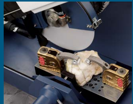
Optional Speed Vise Accessory Kit allows increased flexibility when clamping irregular shapes.
