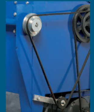
Step pulley allows the operator to change the feed rates.
