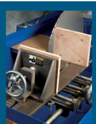
Rock Vise accepts a sample up to 17" (432mm) in size.
