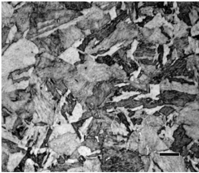
Fig. 4. Carbon-free martensite in 18Ni250 maraging steel (Fe-<0.03% C-18.5% Ni-7.5% Co-4.85% Mo-0.4% Ti-0.1% Al) etched with Fry's reagent (1000x - marker bar is 10 \mu m long)
